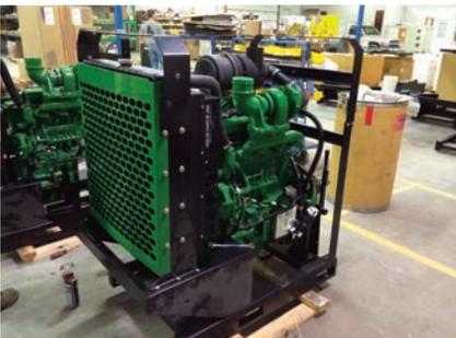
*PowerTech M* engines have 2 valve heads, fixed geometry turbochargers, and mechanical fuel systems. Power Tech M engines are perfect for less demanding applications. Their mechanical controls are simple to operate and maintain.
